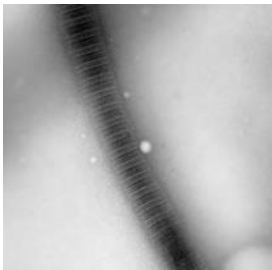
FIGURE 3 - TRANSMISSION ELECTRON MICROSCOPY MICROGRAPH OF NITTA-GEL TYPE I COLLAGEN. [MAGNIFICATION: 10000X]
